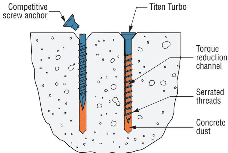
**Patented Torque Reduction Channel
